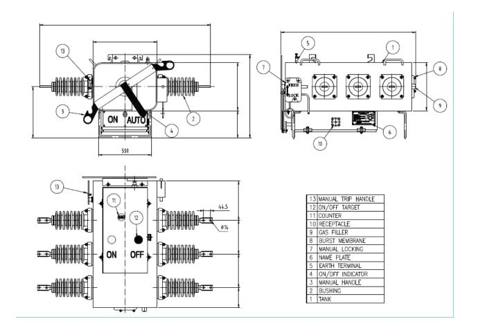
The dimensions in above table are applicable to all the operation types, except for the Manual Type product's height (D). The height (D) of Manual Type Switch is 490 mm regardless of voltage class. And, the dimensions in above table are based on Porcelain Bushing, NEMA Type bare terminal without down-rod ground actuator.
