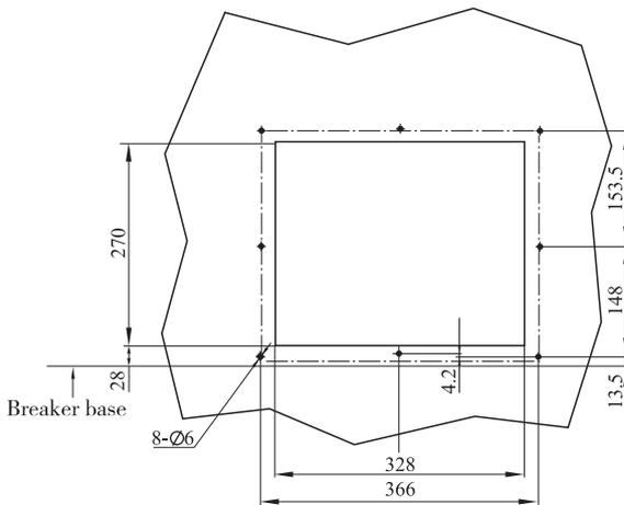
BT3-4000 Intelligent Air Circuit Breaker with four poles (fixed type)
