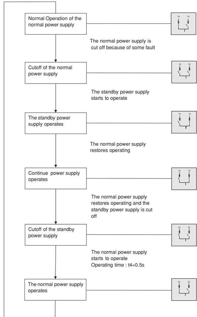
• **Automatic switch with restoration for normal supply from the generation supply (Type F)**
