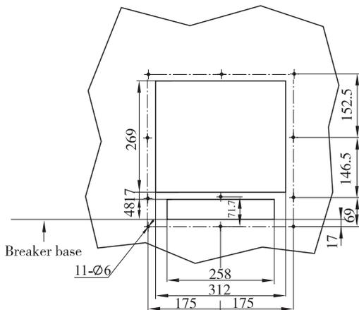
BT3-2500 Intelligent Air Circuit Breaker with four poles (draw-out type)
