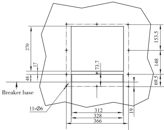
BT3-4000 Intelligent Air Circuit Breaker with four poles (draw-out type)
