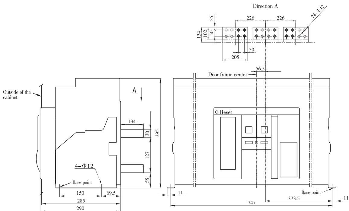
● BT3-6300 Intelligent Air Circuit Breaker with four poles (fixed type)
