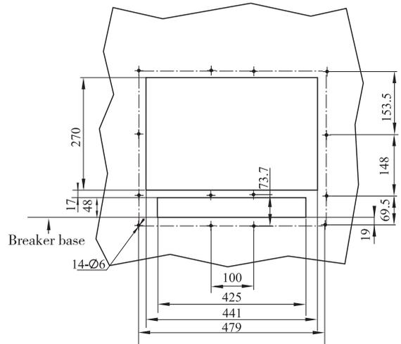
BT3-4000 Intelligent Air Circuit Breaker with three poles (fixed type)
