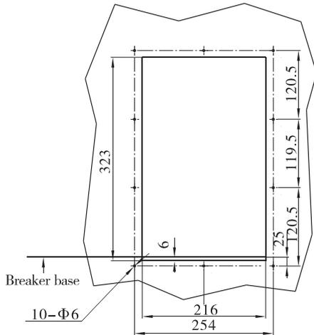
BT3-1600 Intelligent Air Circuit Breaker with four poles (draw-out type)
