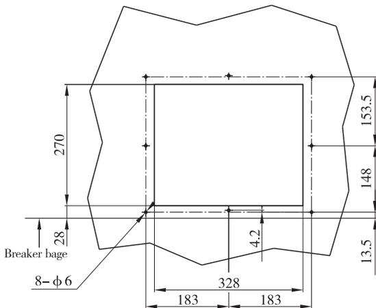
BT3-6300 Intelligent Air Circuit Breaker with four poles (fixed type)
