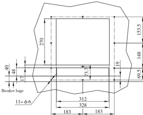
BT3-6300 Intelligent Air Circuit Breaker with four poles (draw-out type)
