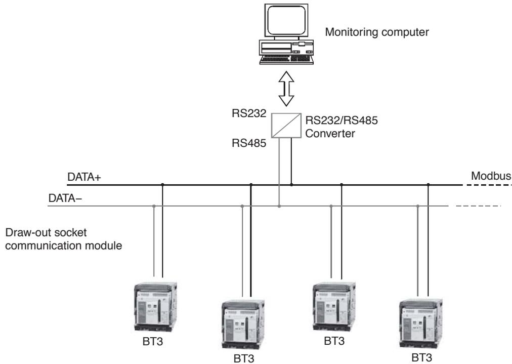
Note: As the accessory of selective purchase, the draw-out socket communication module should be selected into use when users need read the location of main body in the long distance by the choice of draw-out circuit breakers.
