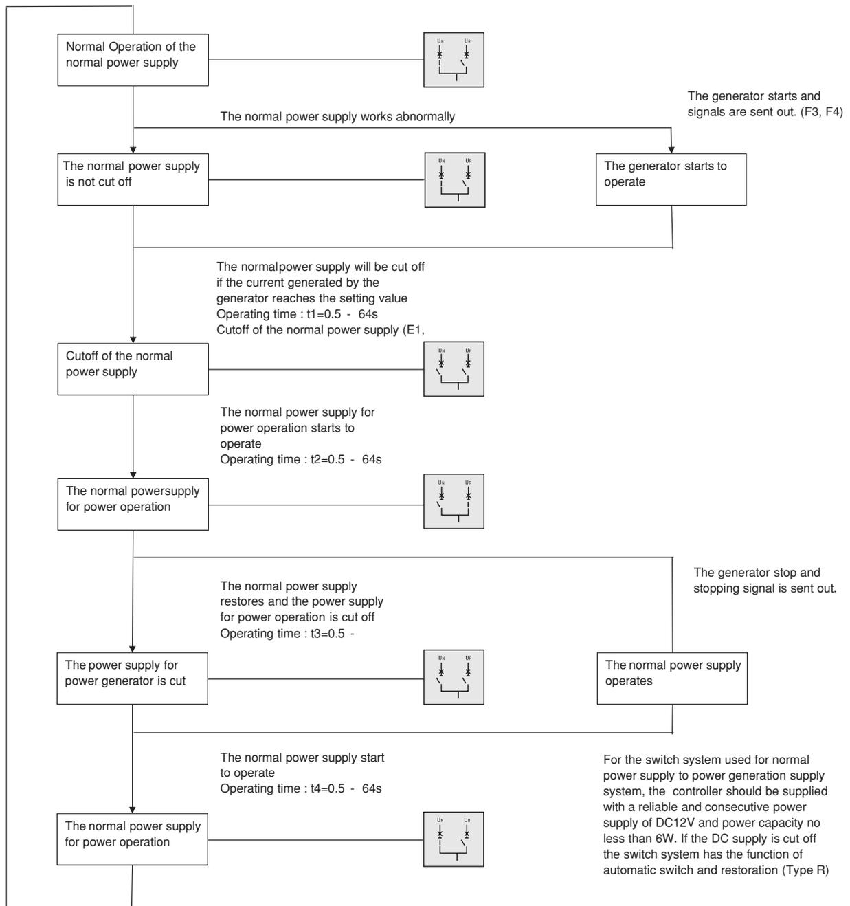
• **Characteristics of the automatic controllers of type R, S and F**
