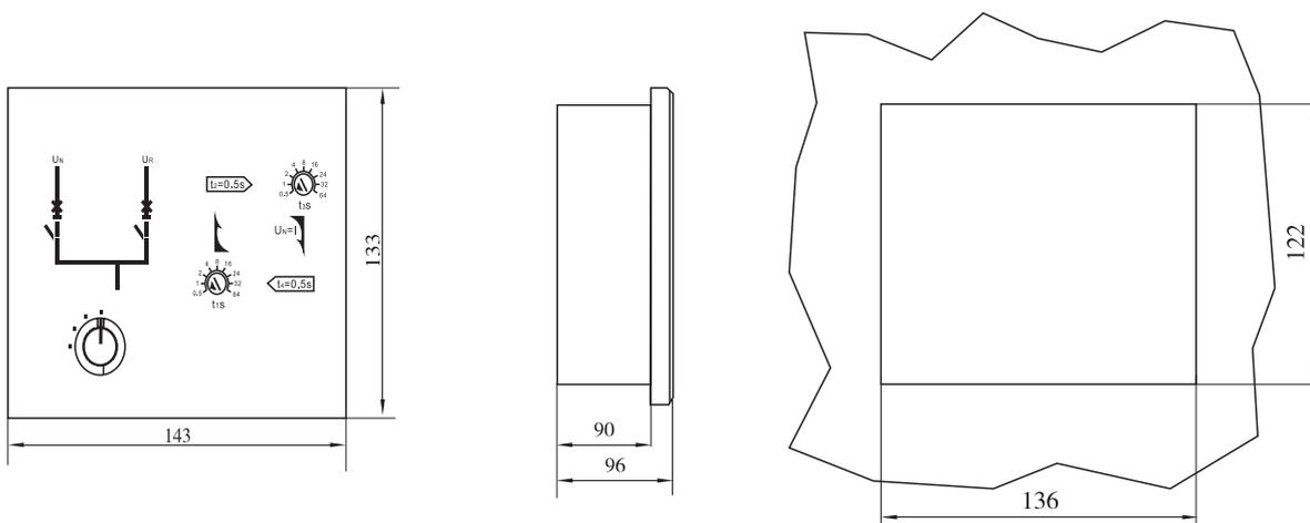
● Automatic power supply switch system of type F
