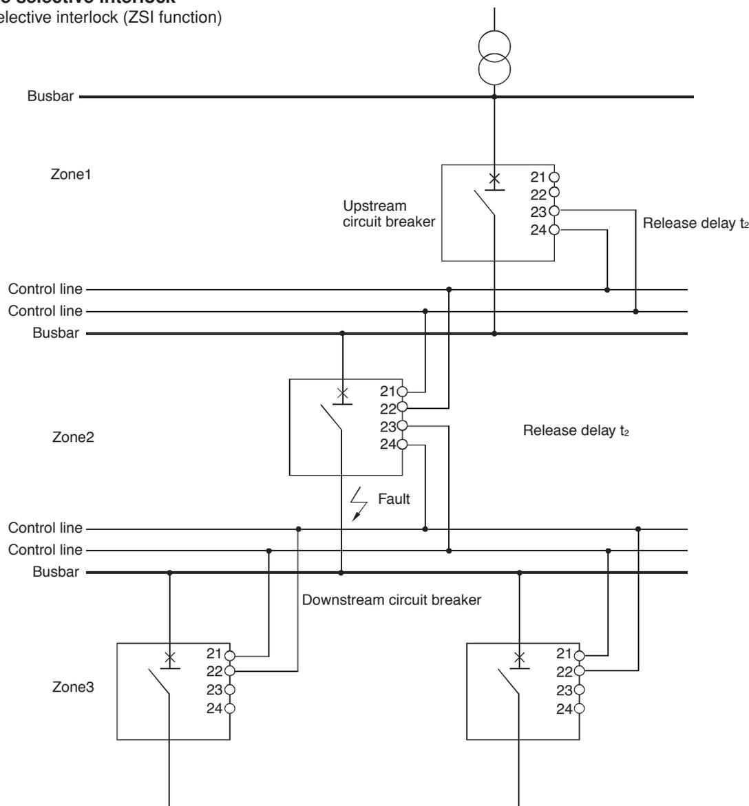
The control circuits are connected to the terminals 21, 22, 23, 24 of the auxiliary terminal
