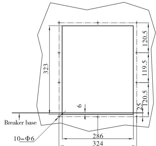
BT3-1600 Intelligent Air Circuit Breaker with three poles (fixed type)
