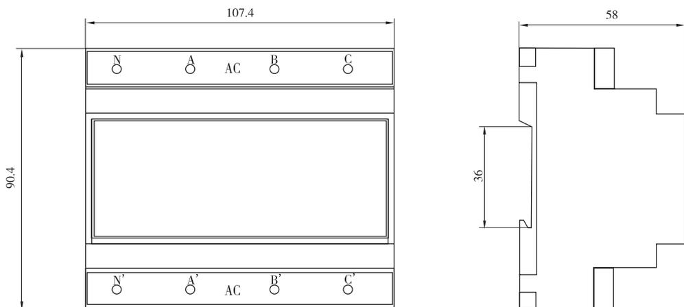
● Delay module of under - voltage release of BT3-1600
