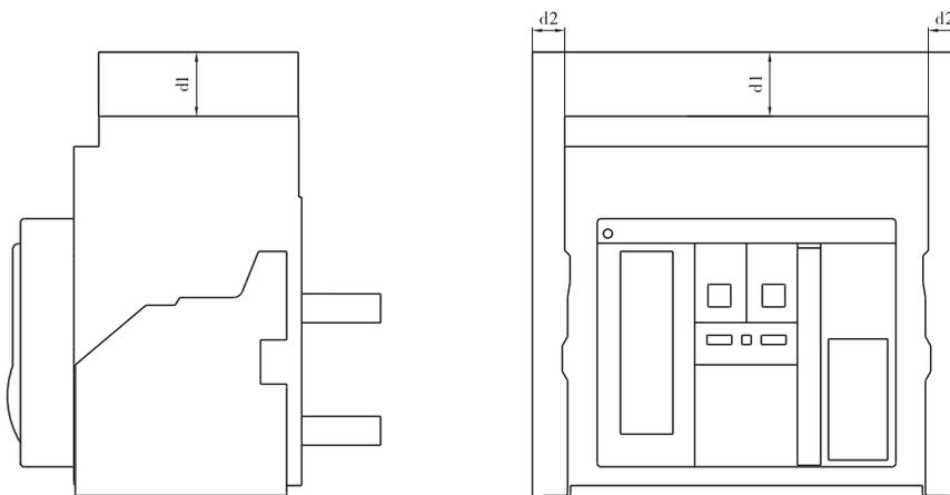
Minimum distance between breakers with switchboard wall or live part.
