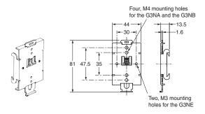
To mount the Relay to DIN
