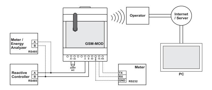
The maximum cable length of RS485 is 1000 meter. If Cable length and number of device is rising you can 120 ohm resistor supplied with device. Connection speed increase with cable length decreases and connection speed decrease with cable length increases. GSM-MOD supports maximum 127 devices.
