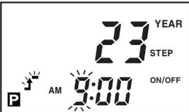
Press **▼** key to set 9 and press **SET** key after check 00min.
