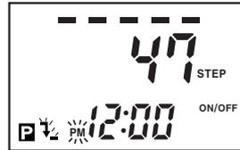
Select PM by **▲** or **▼** keys and move the flashing to hour position by **▶** key.
