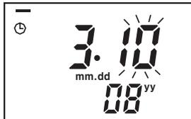
Press **▲** or **▼** keys to set 08 (year 2008) and move the flashing digit to position month by **▶** key. Press **SET** key after press **▲** or **▼** keys to set date 10.
