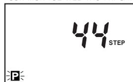
**MODE** key is pressed for 3sec in RUN mode, "P" is flashed and press **SET** key.
