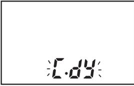
Press **MODE** key over 3sec to move to the setting group1 in RUN mode and press it repeatedly until "L.dY" is flashed in second display part and press **SET** key.
