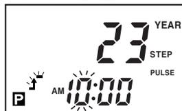
Press **▼** key twice to set 10 and press **SET** key after check 00min.
