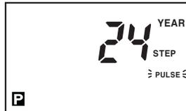
**▲** key is pressed when ON/OFF is flashed to set PULSE mode and press **SET** key.
