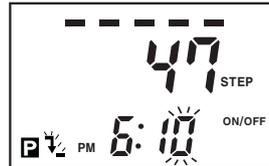
Move the flashing to minute position after set 6:00 by **▲** key and set the minute as 10 and press **SET** key.
