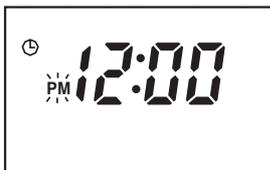
Press **▲** or **▼** keys to select PM and move the flashing digit to position hour by **▶** key.
