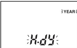
Press **MODE** key over 3sec to move to the setting group1 in RUN mode and press it repeatedly until "H.dY" is flashed in second display part and press **SET** key.
