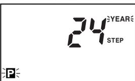
**MODE** key is pressed for 3sec in RUN mode, "PROG P1" is flashed and press **MODE** key again, "PROG P2 YEAR" is flashed and press **SET** key.
