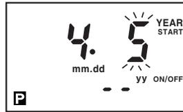
Press **▶** key until month position is flashed and set Apr by **▲** key and press **▶** key until date position is flashed. Press **SET** key after set 5th by **▲** key.
