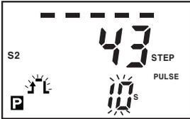
Press **▲** key to select pulse width as 10s(10sec.) and press **SET** key.
