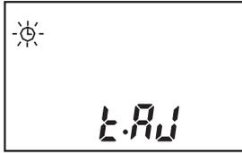
**MODE** + **SET** keys are pressed over 3sec in RUN mode, it is advanced to current time setting of setting group 2 and clock will be flashed and t.AJ will be lighted in second display part, press **SET** key.
