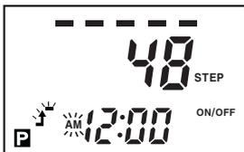
**▶** key is pressed, move the flashing to hour position and select PM by **▲** or **▼** keys when ON time is afternoon.
