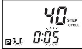
Press **▶** key to move the flashing to minute position and set as 5min by **▲** key and press **SET** key.
