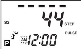
Press **▶** key, move the flashing to hour position and select PM by **▲** or **▼** keys when ON time is afternoon.
