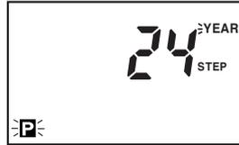
Press **MODE** key for 3 sec in RUN mode, "P" is flashed and press **MODE** key once, then, "P" and YEAR are flashed and press **SET** key to set.
