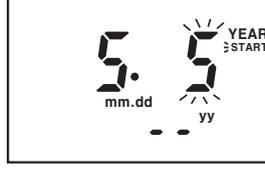
Press **▶** key until month position is flashed and set May by **▲** key and press **▶** key until date position is flashed. Press **SET** key after set 5th by **▲** key.
