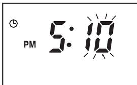
Press **▲** or **▼** keys to set 5 PM and move the flashing digit to position min. by **▶** key. Press **▲** or **▼** key to set 10min and press **SET** key and it is returned to RUN mode when press **MODE** key over 3sec.
