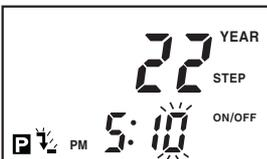
Move the flashing to minute position after set 5 by **▲** key and set the minute as 10 and press **SET** key.
