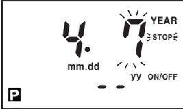
The flashing is moved to month position directly and press **▲** key to set Apr and press **▶** key until date position is flashed.
