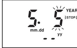
The flashing is moved to month position directly and press **▲** key to set May and press **▶** key until date position is flashed. Press **SET** key after set 5th by **▲** key.
