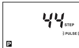
Press **▲** key when ON/OFF is flashed, PULSE is flashed and press **SET** key.
