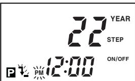
Select PM by **▲** or **▼** keys and move the flashing to hour position by **▶** key.
