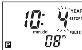
The flashing is moved to month position directly by **▶** key and set 4th by **▲** key after move it to date position by **▶** key, then press **SET** key.
