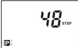
**MODE** key is pressed over 3sec in RUN mode, "P" is flashed and press **SET** key.
