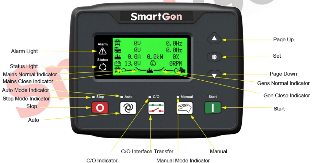
Fig.2 - HGM4020N/HGM4020NC/HGM4020CAN Front Panel Indication
