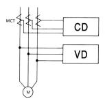
As shown in Fig. 2, open phase is detectable by voltage method without requiring use of a current transformer. The method does not, however, offer ability to detect open phase status between detector contact point to motor. In case of line side open phase, terminal voltage exists if the motor is running with light load that open phase may not be detectable. For this above reason, the current detections method is desirable.
