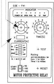
Operating time setting be set from starting to normal operating time (3phase Induction motor)
