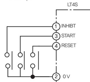
\* LT4S model is non-voltage input type (NPN input)
