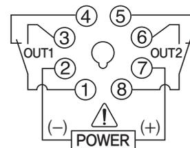
\* When you set CONT to 1c in function setting mode, OUT1 operates as instantaneous output.
