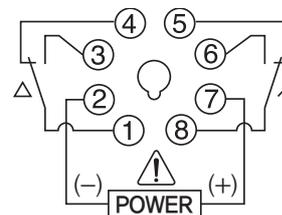
\* When you set O-MD to S-D in function setting mode, OUT1 operates as  $\Delta$  output, and OUT2 operates as  $\wedge$  output.
